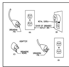
**WARNING**: This heater has a voltage rating of 120 volts. The cord has a plug as shown in A. An adapter as shown in C is available for connecting three-blade grounding-type plugs to two-slot receptacles. The grounding lug extending from the adapter must be connected to a permanent ground such as a properly grounded outlet box. The adapter should not be used if a three-slot grounded receptacle is available.
